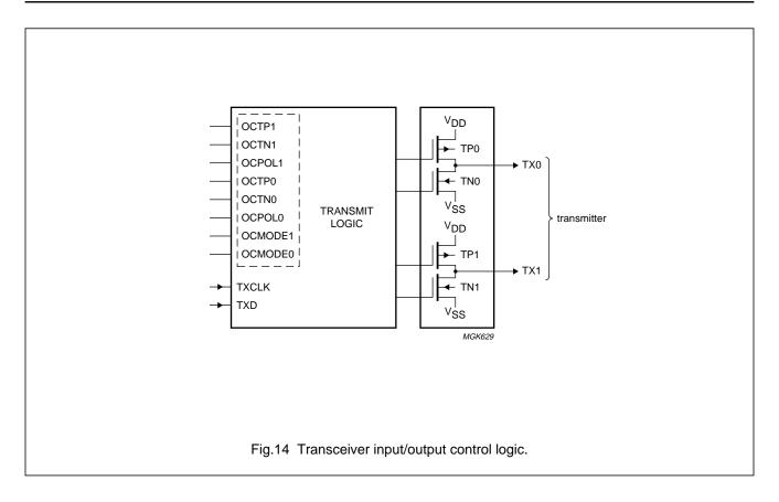
If the SJA1000 is in the sleep mode a recessive level is output on the TX0 and TX1 pins with respect to the contents within the output control register. If the SJA1000 is in the reset state (reset request = HIGH) or the external reset pin RST is pulled LOW the outputs TX0 and TX1 are floating.
