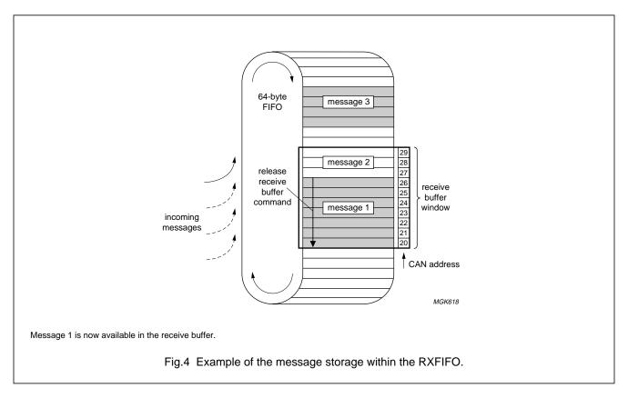
Identifier, remote transmission request bit and data length code have the same meaning and location as described in the transmit buffer but within the address range 20 to 29.
